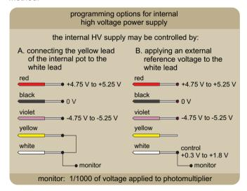
When using the internal pot the photomultiplier tube high voltage is increased by clockwise rotation. Monitor the photomultiplier tube high voltage with a voltmeter connected between the white (control) and black (0V) wires. The photomultiplier tube voltage is 1000 x the voltage on the control (white) wire. Take care not to exceed the maximum rated voltage for the photomultiplier tube, as specified in the module test data
