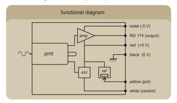
The internal high voltage supply to the photomultiplier tube can be controlled used the internal pot, accessed from the back face of the module, or by applying an external control voltage. Make connections to the yellow (pot) and white (control) wires, as shown in the table below, according to your choice of control method
